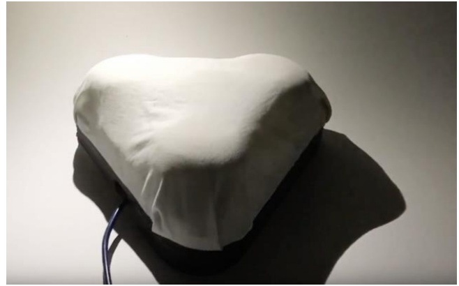
Figure 5. The physical artifact: beneath the cushion-like cover there are four hidden buttons and an Arduino. The cable running from the controller connects to a computer.
